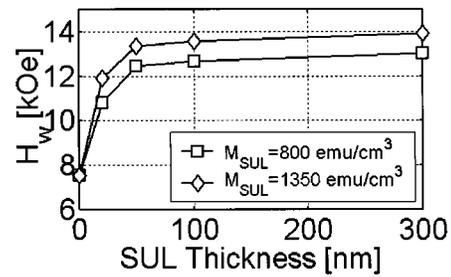
Fig. 7. Maximum magnitude of  $H_w$  as a function of SUL thickness for SUL magnetization of 800 and 1350 emu/cm<sup>3</sup>.
