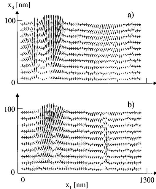
Fig. 4. Soft underlayer magnetization for  $d_{\text{SUL}} = 100$  nm. (a)  $M_{\text{SUL}} = 800$  emu/cm<sup>3</sup>. (b)  $M_{\text{SUL}} = 1350$  emu/cm<sup>3</sup>.
