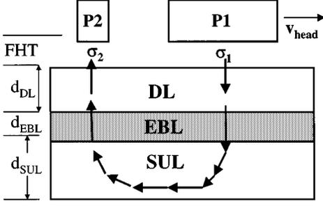
Fig. 1. Model geometry showing magnetic flux flowing through the SUL.
