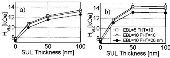
Fig. 8. Maximum magnitude of  $H_w$  as a function of  $d_{SUL}$  for  $P2 = 320 \times 320 \text{ nm}^2$ . (a)  $M_{SUL} = 800 \text{ emu/cm}^3$ . (b)  $M_{SUL} = 1350 \text{ emu/cm}^3$ .
