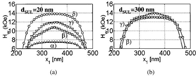
Fig. 6. Field profiles for (a)  $d_{\text{SUL}} = 20$  nm and (b)  $d_{\text{SUL}} = 300$  nm; ( $\alpha$ ) without SUL contributions, ( $\beta$ )  $M_{\text{SUL}} = 800$  emu/cm<sup>3</sup>, ( $\gamma$ )  $M_{\text{SUL}} = 1350$  emu/cm<sup>3</sup>, ( $\delta$ ) perfect imaging.
