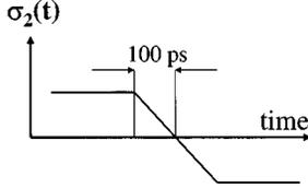
Fig. 2. Temporal profile of the charge density on P2.
