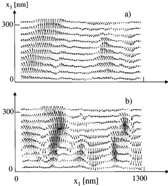
Fig. 5. Soft underlayer magnetization for  $d_{\text{SUL}} = 310$  nm. (a)  $M_{\text{SUL}} = 800$  emu/cm<sup>3</sup>. (b)  $M_{\text{SUL}} = 1350$  emu/cm<sup>3</sup>.
