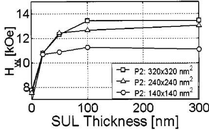
Fig. 9. Maximum field  $H_w$  as a function of  $d_{SUL}$  for three head sizes at  $M_{SUL} = 800 \text{ emu/cm}^3$ .
