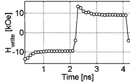
Fig. 12. Time dependence of the total write field during writing of a 40-nm dibit.
