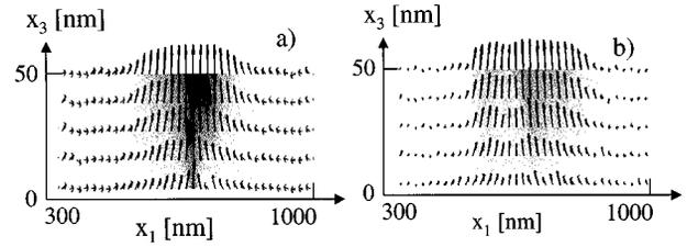
Fig. 11. Magnetization in the SUL below P2 for  $d_{SUL} = 50 \text{ nm}$ . (a)  $H_{k,SUL} = 10 \text{ Oe}$ . (b)  $H_{k,SUL} = 3840 \text{ Oe}$ .
