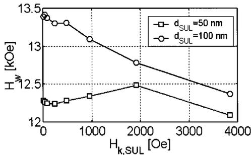
Fig. 10. Maximum  $H_w$  as a function of SUL anisotropy field for  $d_{SUL} = 50 \text{ nm}$  and  $d_{SUL} = 100 \text{ nm}$ .
