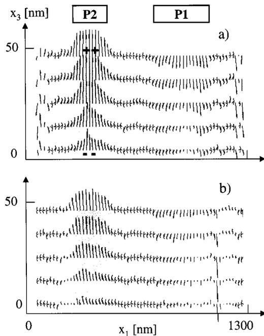
Fig. 3. Soft underlayer magnetization for  $d_{\text{SUL}} = 50$  nm. (a)  $M_{\text{SUL}} = 800$  emu/cm<sup>3</sup>. (b)  $M_{\text{SUL}} = 1350$  emu/cm<sup>3</sup>.
