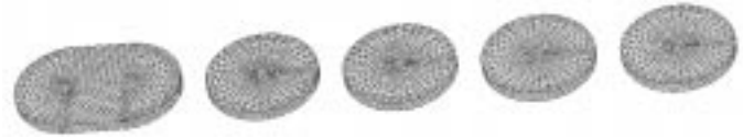
Fig. 1. Finite element model of a chain of circular nanodots. The surface mesh used for the boundary element method is given as a wireframe.
