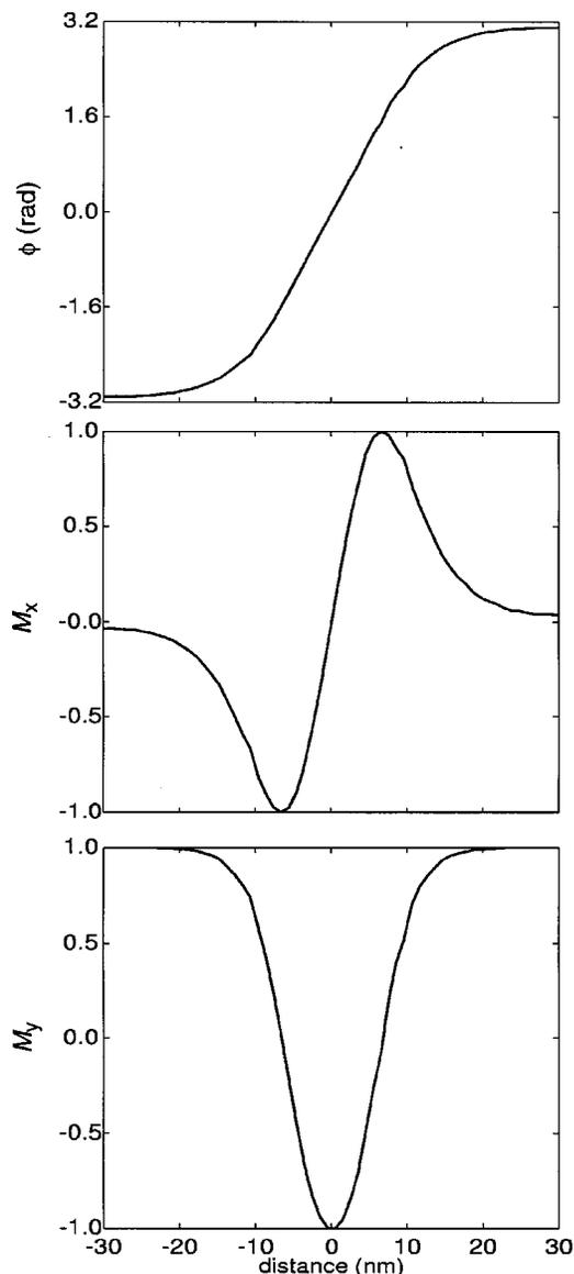
FIG. 3. Profile of the horizontal  $360^\circ$  wall. The plots give the angle of the magnetization with respect to the  $y$  axis, the  $x$  component of the magnetization, and the  $y$  component of the magnetization as a function of distance along a line parallel to the  $y$  axis.
