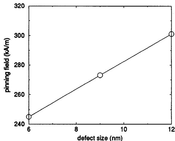
FIG. 4. The external field required to eliminate the  $360^\circ$  wall structure as a function of the size of the nonmagnetic defect.
