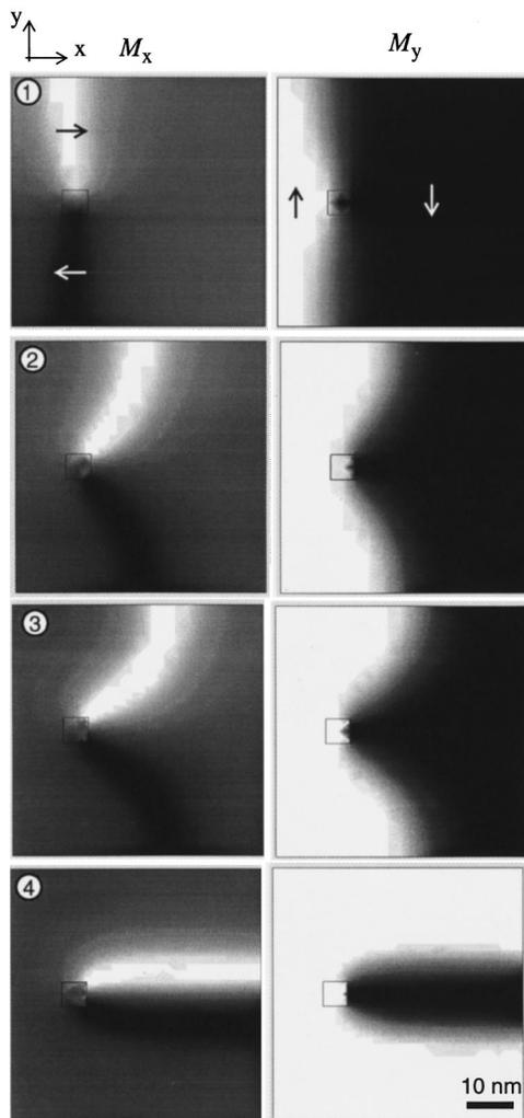
FIG. 1. Simulation of the formation of a 360° domain wall in a thin Co film. An external field of  $H_{\text{ext}}=160$  kA/m is applied in the positive  $y$  direction. The gray scale plots of the left and right columns depict the  $x$  and  $y$  components of the magnetization, respectively. The numbers refer to the finite element grids presented in Fig. 2.
