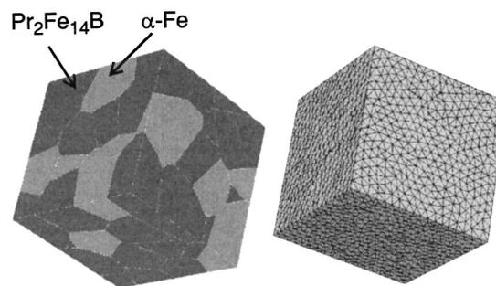
FIG. 1. Model of the nanocomposite magnet used for the simulation. The gray regions correspond to soft magnetic  $\alpha\text{-Fe}$  grains, the black regions denote hard magnetic  $\text{Pr}_2\text{Fe}_{14}\text{B}$  grains. The total number of grains is 64. The figure on the right hand side shows the triangulation of the grains into finite elements.
