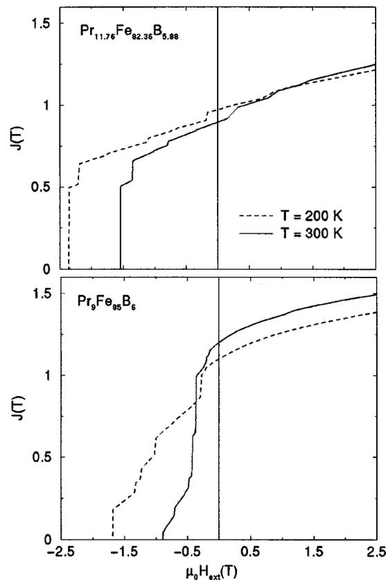
FIG. 3. Calculated demagnetization curves for the single-phase Pr<sub>11.76</sub>Fe<sub>82.36</sub>B<sub>5.88</sub> and the two-phase  $\alpha$ -Fe/Pr<sub>2</sub>Fe<sub>14</sub>B magnet at 200 and 300 K.
