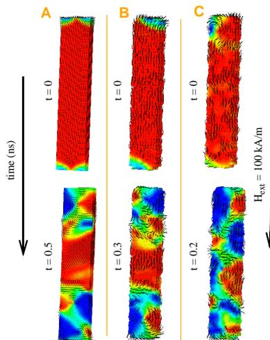
Remanent states and transient states during the magnetization reversal of 80 nm x 400 nm x 25 nm Co elements.
