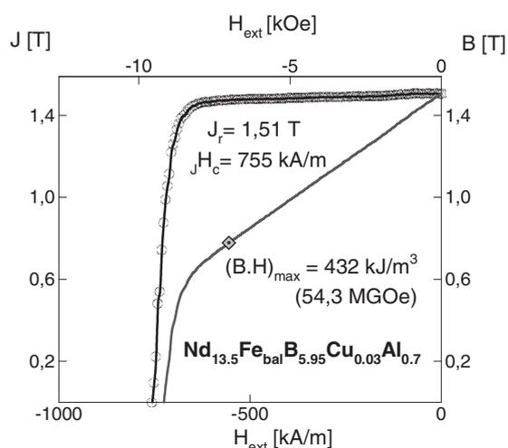
**Figure 5.** The demagnetization curve of an optimized high energy density sintered magnet manufactured using a combination of a rubber isostatic die and TDP.
