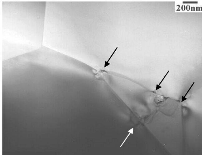
**Figure 6.** A TEM image of grain boundary junctions of a  $\text{Nd}_{13.7}\text{Fe}_{\text{bal}}\text{B}_{5.95}\text{Cu}_{0.03}\text{Al}_{0.7}$  sintered magnet with the  $c$ -axis of the grains perpendicular to the image plane. Pockets of Nd-rich phases are marked by arrows.
