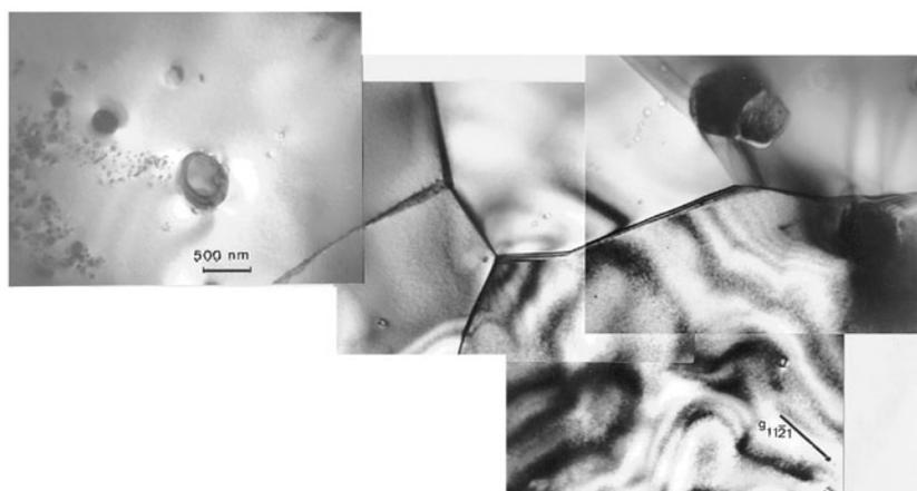
**Figure 2.** A TEM micrograph of a sintered  $\text{SmCo}_5$  magnet showing several grains containing  $\text{Sm}_2\text{O}_3$  and  $\text{CaO}$  inclusions. The coercivity mechanism is controlled by the nucleation and expansion of reversed domains.
