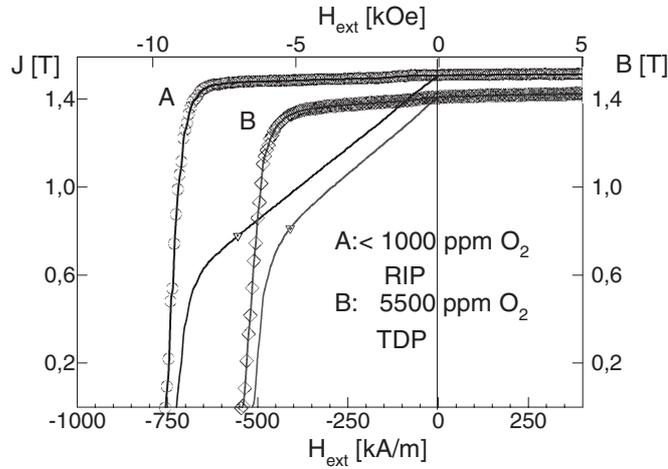
**Figure 4.** Comparison of demagnetization curves of  $\text{Nd}_{13.5}\text{Fe}_{61}\text{B}_{5.95}\text{Cu}_{0.03}\text{Al}_{0.7}$  sintered magnets manufactured by rubber isostatic die pressing and transverse die pressing (TDP) in air; (A)  $J_r = 1.45$  T,  $(BH)_{\max} = 50.2$  MGOe, (B)  $J_r = 1.41$  T,  $(BH)_{\max} = 41.9$  MGOe.
