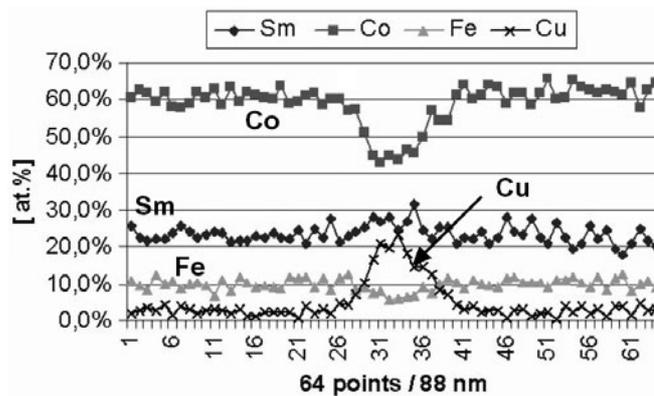
**Figure 9.** Elemental TEM nanoprofile profiles across a cell boundary phase.
