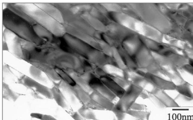
**Figure 3.** A TEM micrograph of a hot pressed and die-upset Nd<sub>14</sub>Fe<sub>72</sub>Co<sub>7</sub>B<sub>6</sub>Ga<sub>1</sub> magnet.
