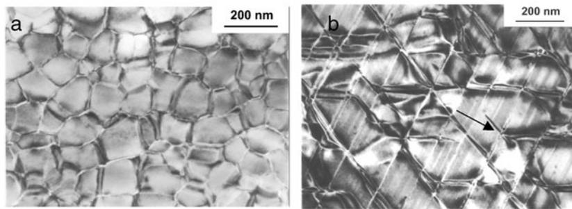
**Figure 8.** TEM micrographs showing typical, rhombic, cellular precipitation structures of a sintered  $\text{SmCo}_5/\text{Sm}_2\text{Co}_{17}$  magnet for high temperature applications. Views (a) parallel and (b) perpendicular to the alignment direction ( $\rightarrow$ ).
