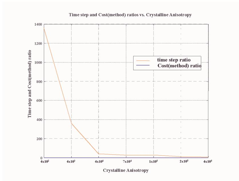
Figure 1: Stiffness ratios vs. Crystalline Anisotropy.
