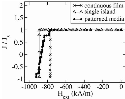
Figure 2 Calculated demagnetization curves for the granular film, patterned media, and a single island.
