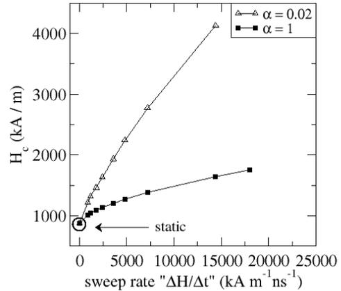
Figure 5 Dynamical coercivity as a function of the field sweep rate for two different values of the damping constant  $\alpha$ .
