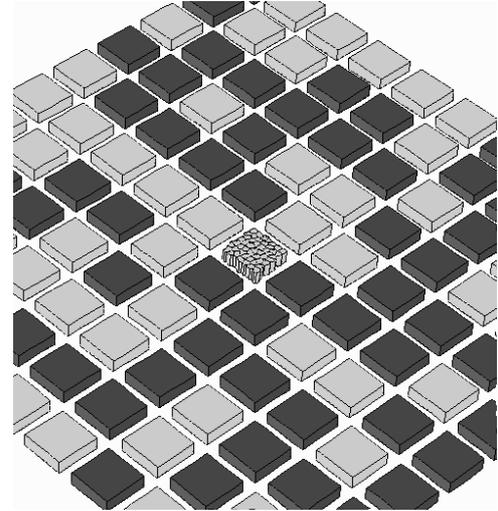
Figure 3 Array of 121 islands as a model for patterned media. The magnetization is set random, representing the written state of a hard disk.
