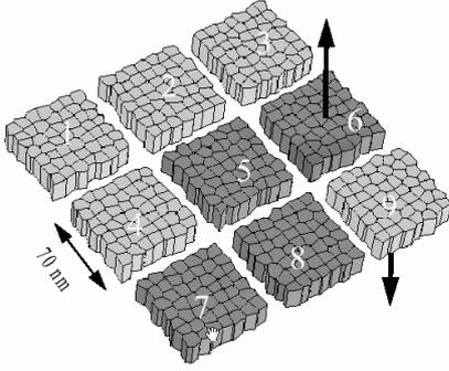
Figure 1 Islands of the discrete media at an external field of  $-870$  kA/m. Bright: Magnetization down; dark: Magnetization up.
